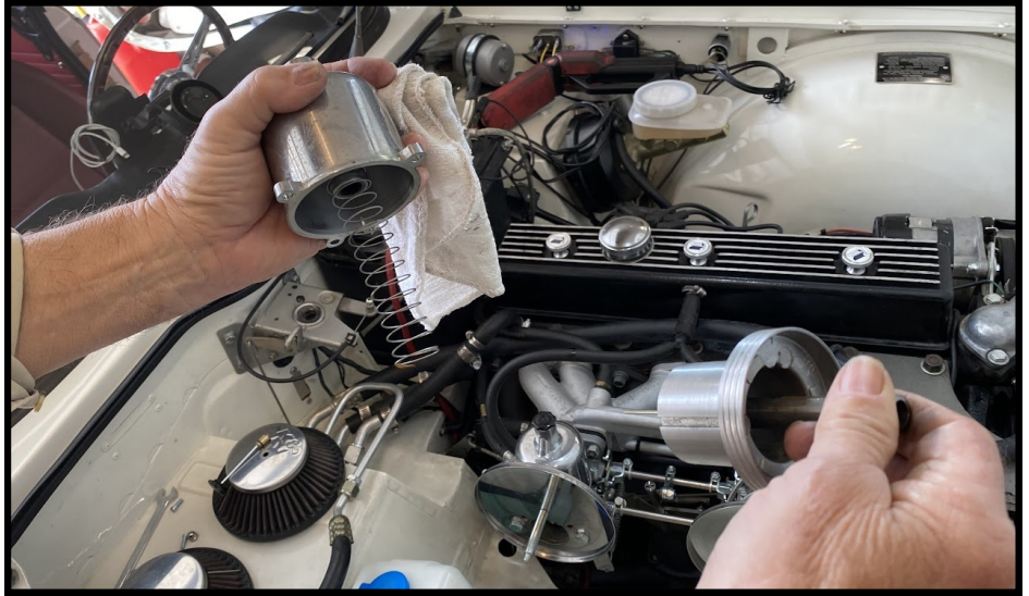
Damper removed, looking at the piston
