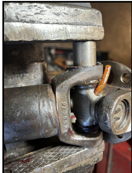
Using a socket for the final push
