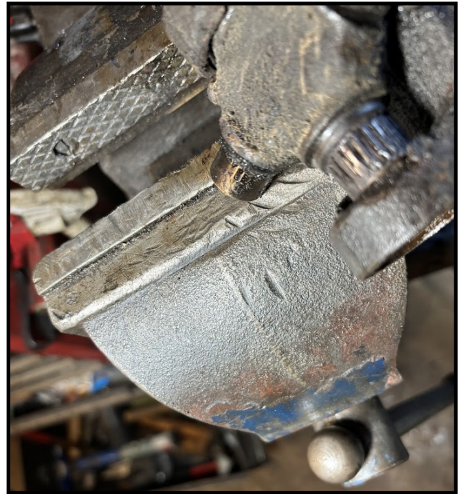
Badly damaged spider
