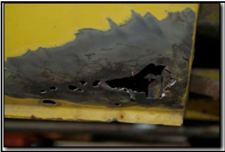
Perforated rust spot
