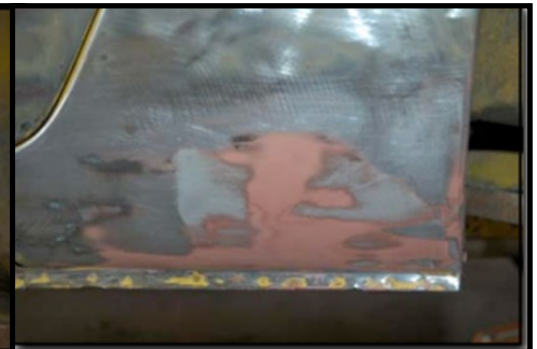
Body putty; glazing; sanding; ready for paint
