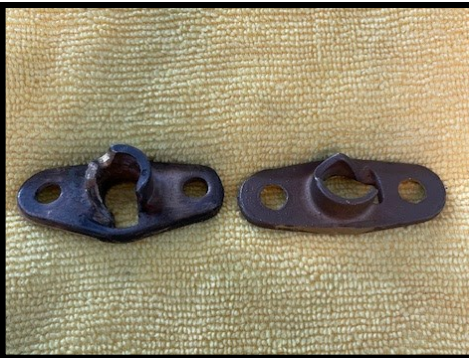
Underside of latching plates. Plate on the left - original. Plate on the right - Rimmer Bros.
