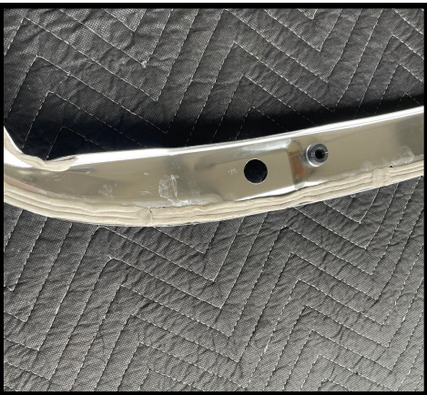
Backside of a new windshield frame cap. Caulk Cord Weatherseal is applied on the front edge.
