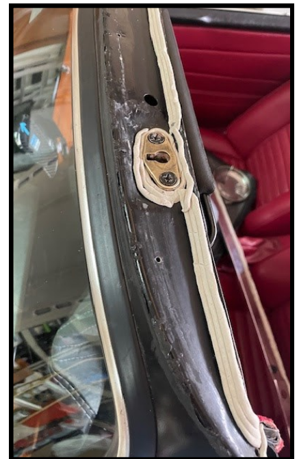
Top of windshield frame with latch in place and caulk cord weatherseal applied.
