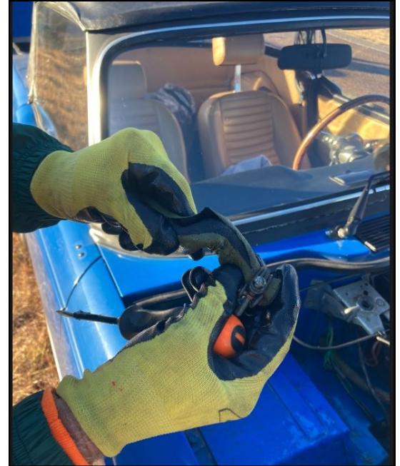
Benson's split heater hose
