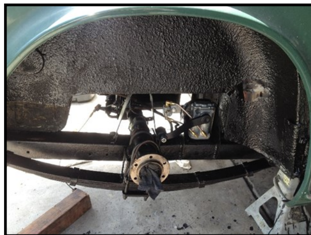
Figure 1: Triumph axle 'as found' before conversion
