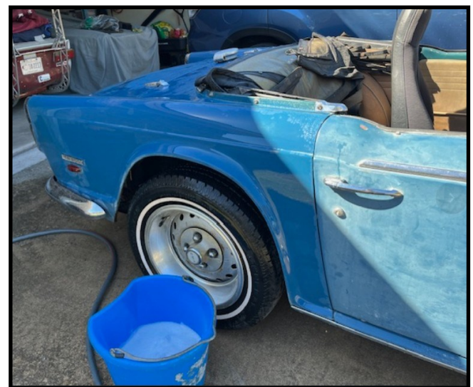
Cleaning up, clay bar, and buffing out the oxidation
