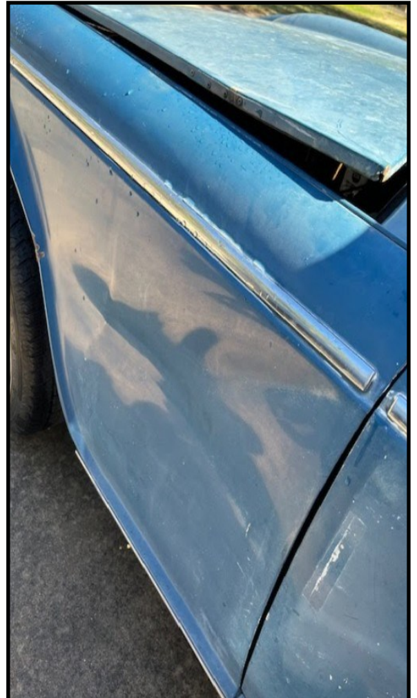
Significant crease in the driver's side front panel
