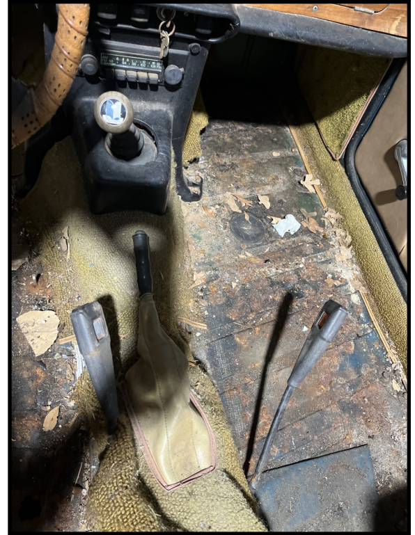
Floorpans after uncovering. They are now cleaned up and patched
