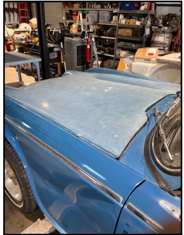
Significant oxidation on the bonnet -- now remediated
