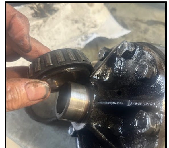
Carrier bearing falling off assembly
