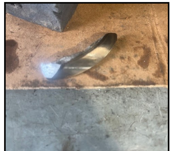
Tooth broken off of Jacques’ pinion gear
