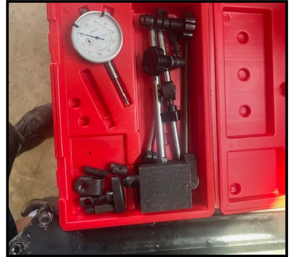
Tools of the trade. Dial indicator for setting backlash
