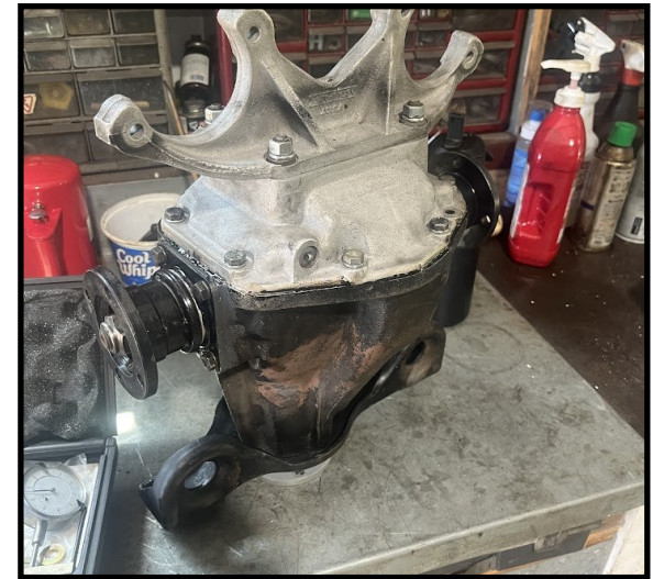
Jacques' rebuilt differential ready for paint
