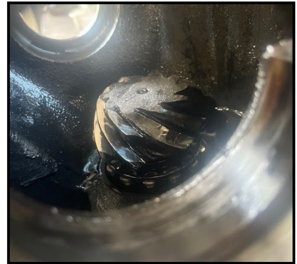
More “ouch” from Jacques’ car - broken pinion gear
