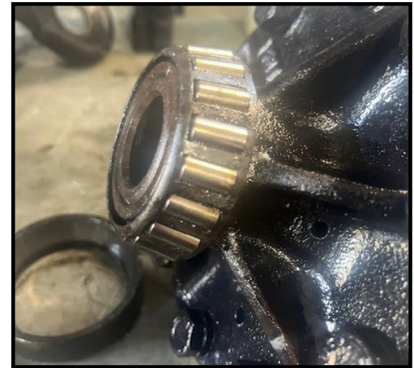
Spun carrier bearing. Picture 1 shows it in place
