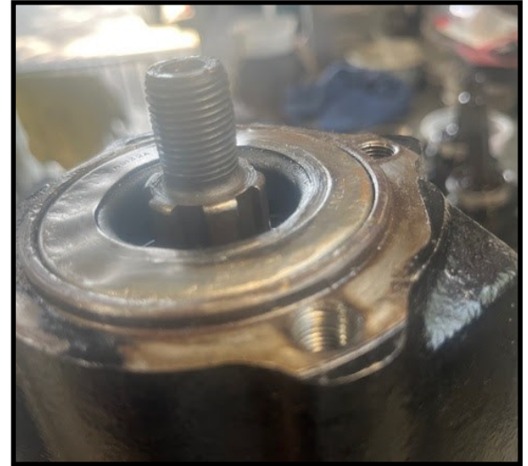
What not to do. Seal hammered, not pressed, into place.
