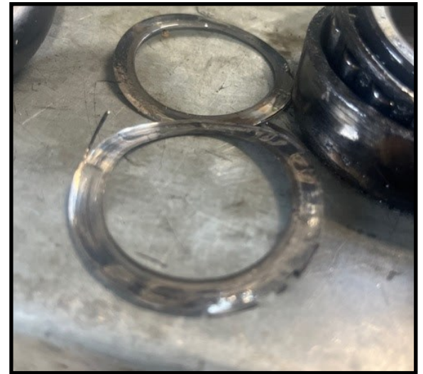
Carrier bearing shims showing effects of spinning
