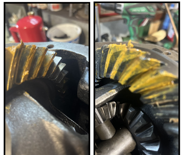
1st pic teeth are too close to the edge; Fixed in 2nd pic
