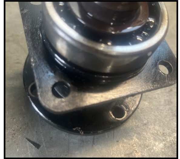
Side seal covers had no sealant
