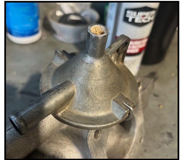
TR4 PCV valve with hose barb cut off
