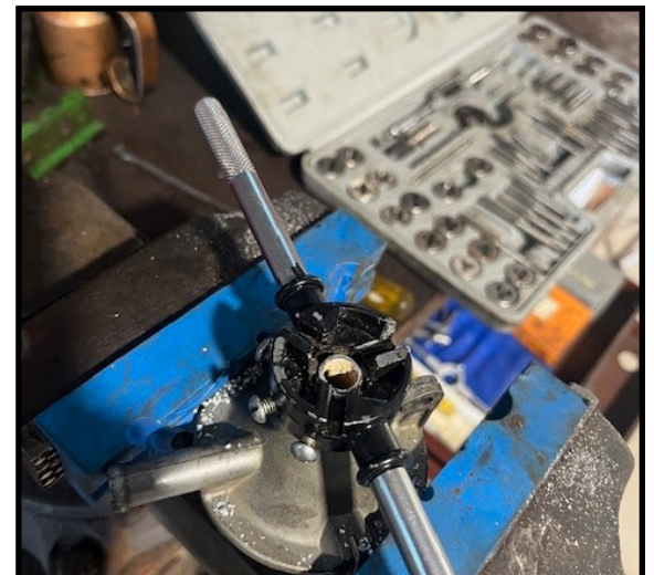
Threading the modified PCV valve
