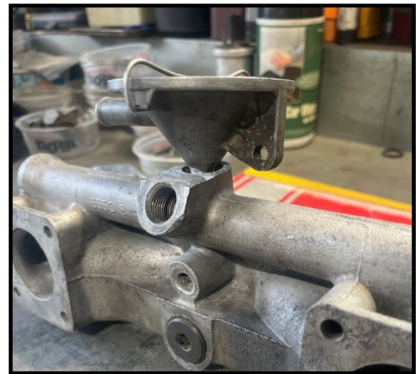
PCV valve threaded into manifold
