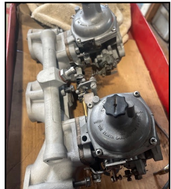
Post-1971 Carbs with side ports for carbon canister
