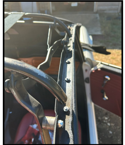
Kit in place, channel & channel seals set
