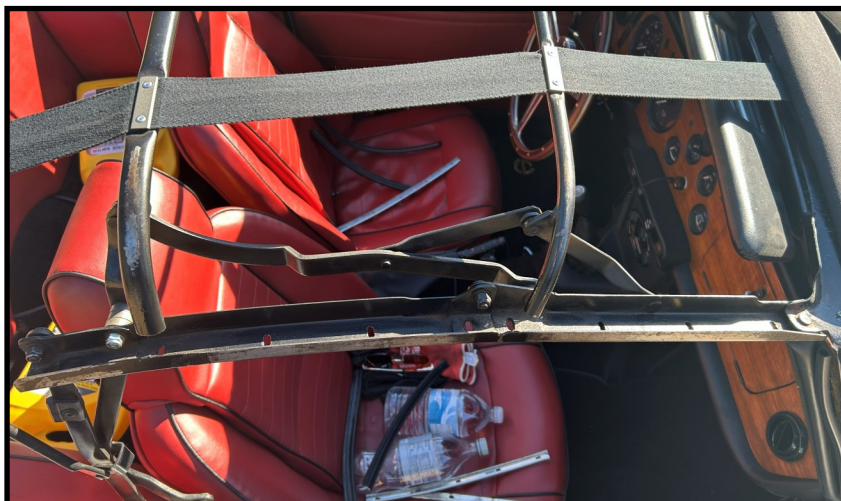
Top frame with top side rails; nuts, washers; and bolts & top side seals removed. Parts removed can be seen on both passenger and driver's seat.
