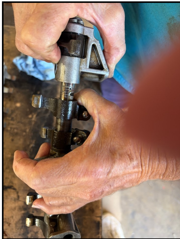
Wear on the rocker shaft
