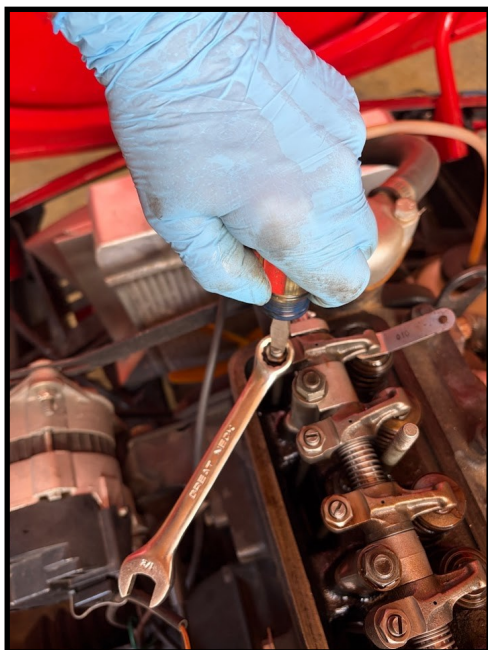
Adjusting the #1 exhaust valve
