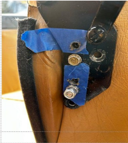
Drilling out new holes
