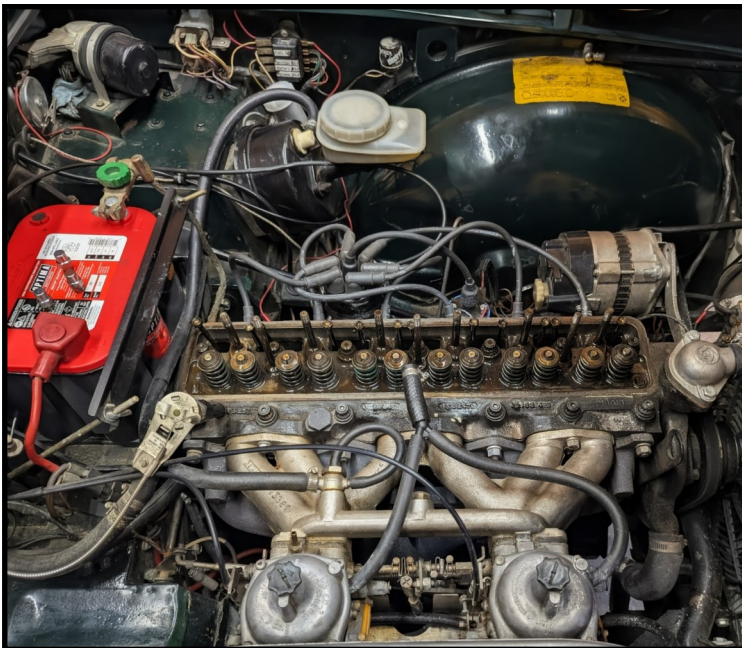
Valve cover off and ready to replace the rocker assembly
