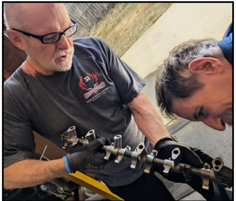
Mike handling the new rocker assembly prior to installation
