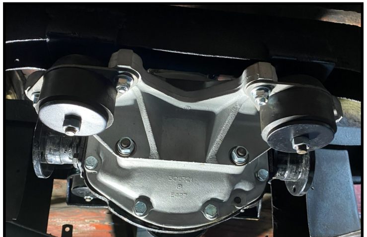
Mounts boxed in and differential remounted to the chassis
