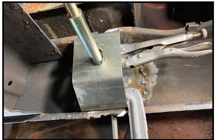
Replacing the mount prior to 'boxing' it in
