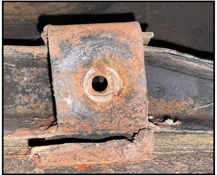
Broken differential mount
