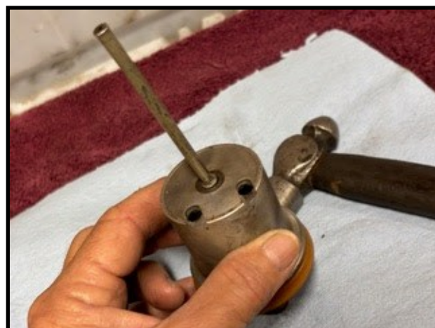
Knocking out the needle
