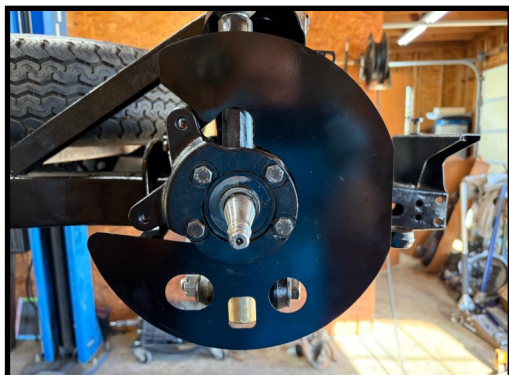
Hub goes on the spindle
