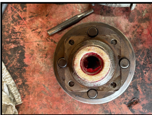
Set the seal with a punch
