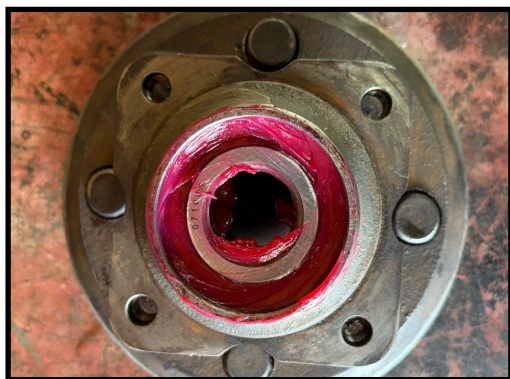
Packed with grease
