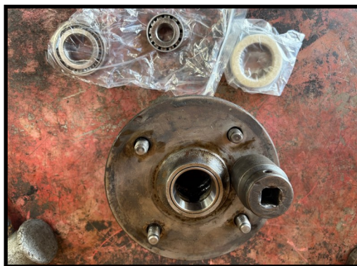
Press it with a socket ...
