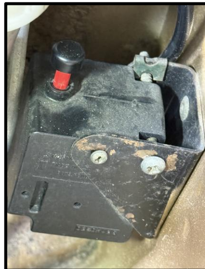
Inertia switch for fuel control
